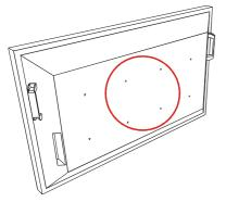
• Take the table stand and attach its mounting plate to the rear of the monitor using the previously removed screws and washers.
